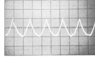
6 .5 V/cm, 2 ms/cm (LOOP OPEN, FREQ ERROR 50 parts in 10^{10} )
